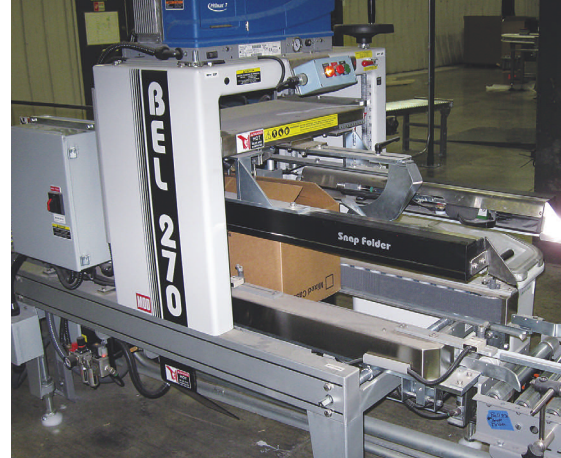
Stacks of cartons are manually loaded into shippers after which they are conveyed to a hot-melt top sealer.
